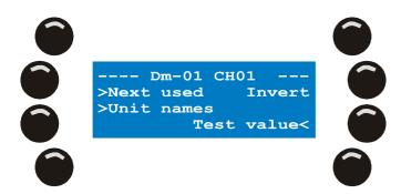
The main LCD indicates that we are editing the logical channel with name CH01 of dimmer unit 01.
