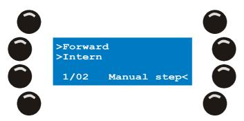
Xciter starts running the sequence. The scene counter on the bottom left indicates the current step. From this point on you have several options to run the sequence.
