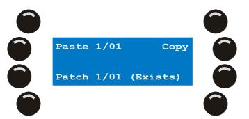
Use page keys 1-8 and general-purpose number keys 1-20 to select patch 102. In our example patch 102 is empty. Press {Paste 1/01} to paste the clipboard content into patch 102. Patch
