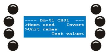
The main LCD indicates that we are editing the logical channel with name CH01 of dimmer unit 01.
