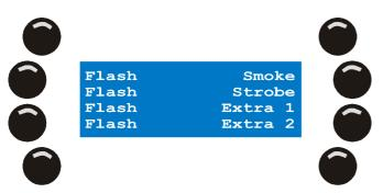
2. Press the softkey to the right of the DA button you wish to edit. **Example:** {Smoke}. Xciter shows a dialog on LCD2 that looks a lot like the dimmer soft patch.
